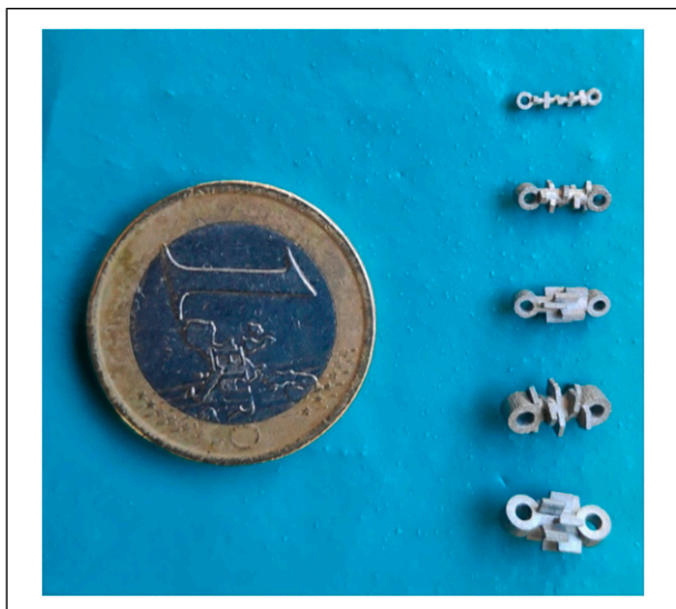
Figure 3. Cylindrical curettes 3D printed from surgical steel.
